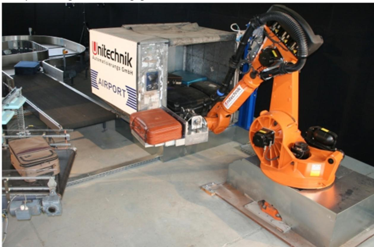
Automated baggage loading: The robot's patented 'gripper' is developed to increase performance and efficiency of the loading process.
