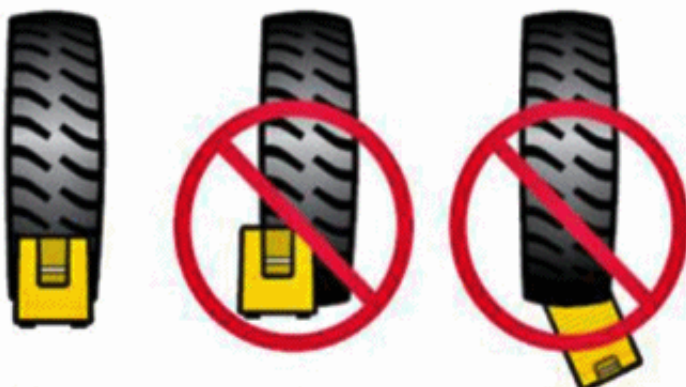
Place chock in the center and square to tire.
